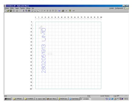
As you can see in this graphic, the message is composed by the date 280205 (without spaces between the numbers), then the hour 1913 and finally the message that comes from the thickness detector (Stil UM0) which can be an A (piece Accepted) or a R (piece Rejected).
